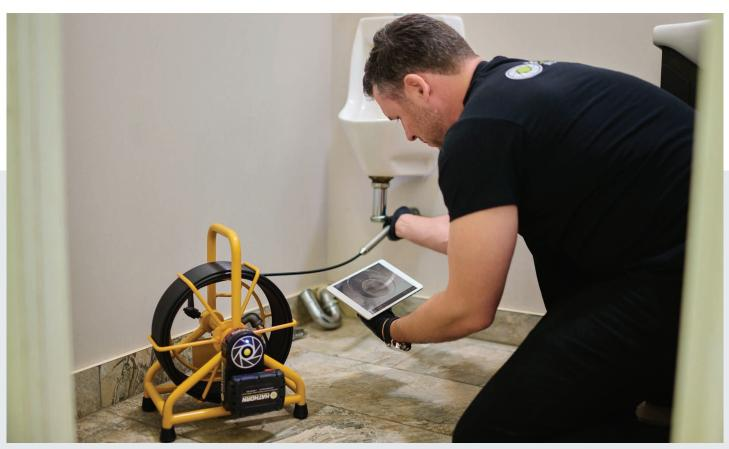
Micron camera reels can be used with either Hathorn® control modules (H12+ recommended), or with your own mobile Apple/Android device, should you opt for the Wi-Fi option. The Wi-Fi option is a standalone camera system that allows live streaming and recording to up to three devices at the same time using Hathorn's free app. It is powered by an external Milwaukee® 18V or equivalent battery (sold separately), which can last over 12 hours.
